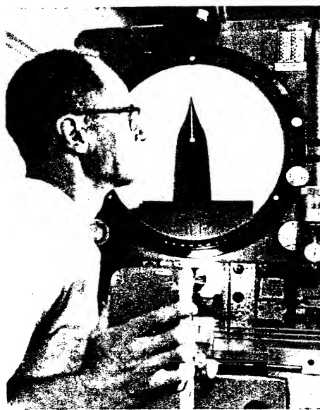
Ernest Skinner (Inspection) checks the shape of a sample pen point which has been magnified 10 times on this contour projector screen in order to permit closer inspection of the nib. This is only one of the many inspections which Sheaffer products undergo before leaving the factory.
